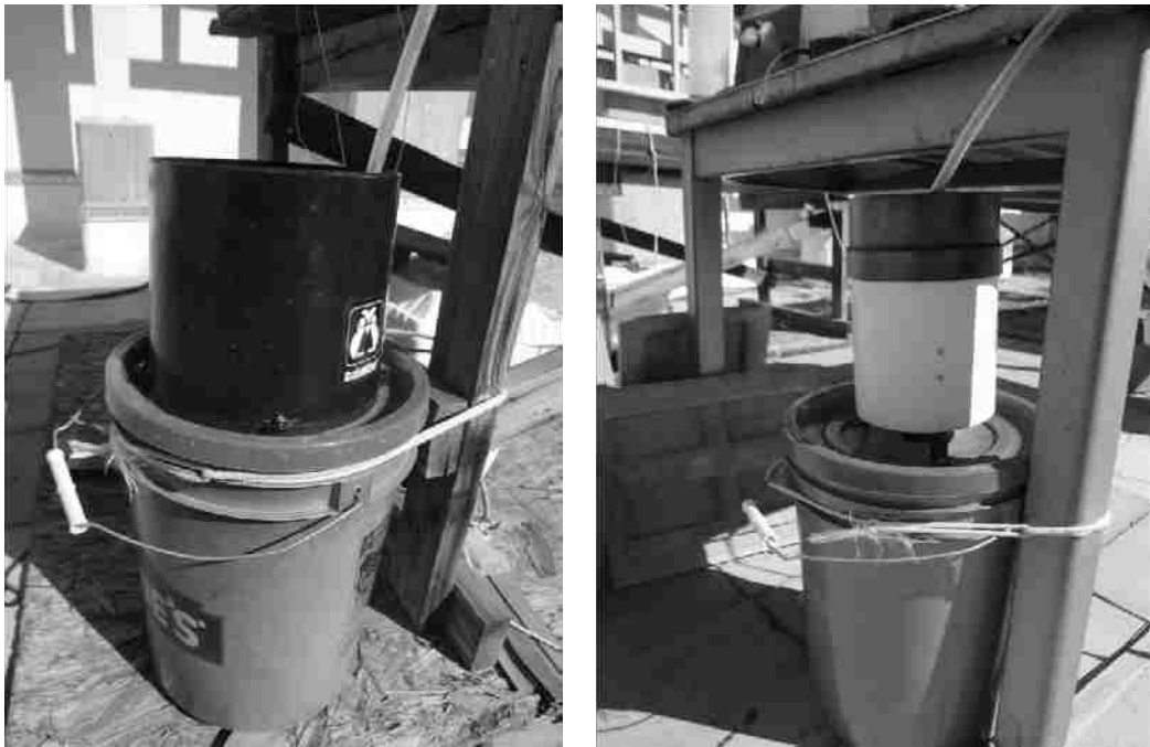
Figure 2.8 Rainwise (left) and Onset (right) rain gauge data loggers attached to SS1-A and SS1-B, respectively
